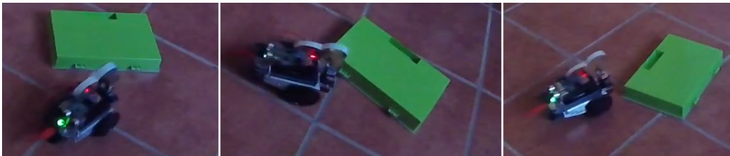
Figure 19. Exercise of avoiding obstacles by visual depth estimation in PiBot
