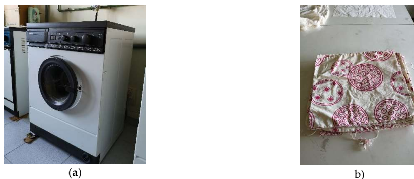
Figure 3. Image of the experimental setup for washing cycles test. (a) Used washing machine (b) Support fabric for washing cycles.
