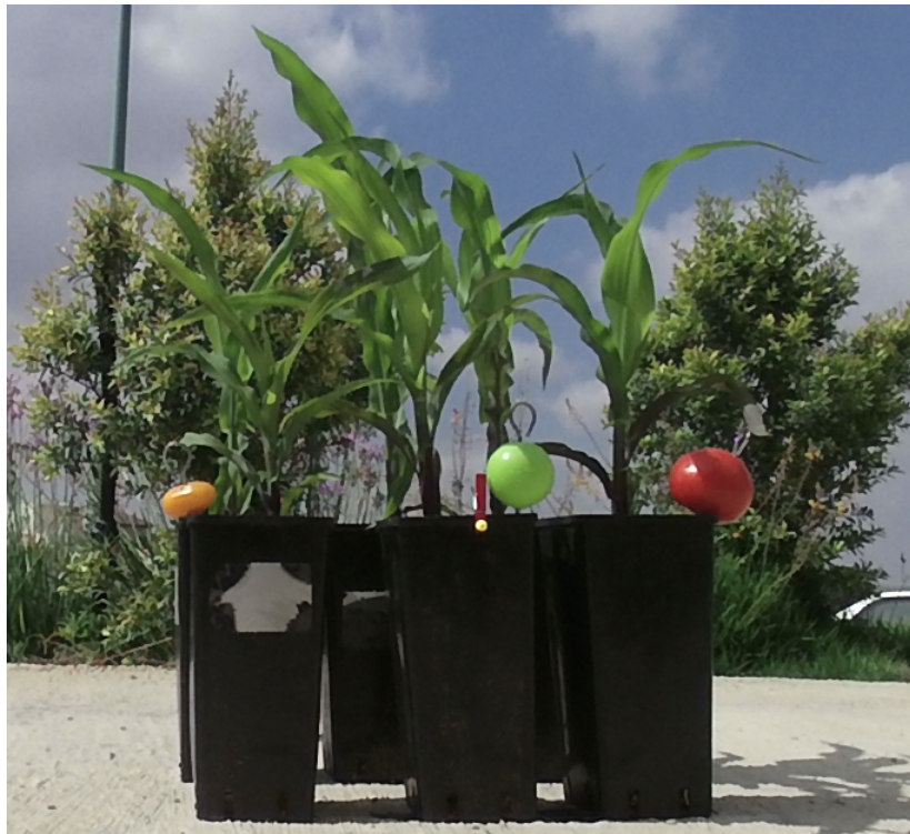
Figure 2. The experimental setup as captured by the Kinect sensor from 1 meter. Six corn plants in black plastic pots arranged in two rows. Added tomatoes — a red tomato, an orange cherry tomato. Two plastic balls for size measurements — a larger green ball and a smaller yellow ball.
