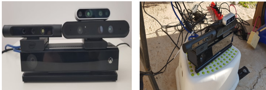
Figure 1. The setup of the 4 sensors used in the experiment. Kinect II at the bottom, the Astra Pro on the left, the SR300 on the right, and the gray D435 on top of the SR300.
