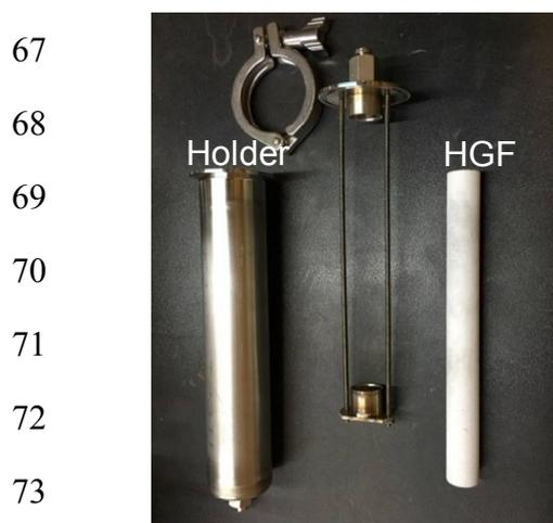
74 **Figure 1.** Schematic pictures of CHGF: Hot gas filtration holder and the filter (left); Packed bed of
