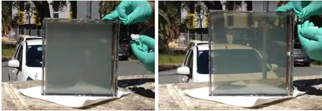
Figure 5. Transparency-controlled, self-powering PDLC-integrated “smart” solar window demonstration at Edith Cowan University (ECU) in Oct. 2014. A 200mm × 200mm hybrid concentrator-type solar window used four parallel-connected edge-mounted CuInSe 2 modules of size 198mm × 25mm, the electric output of which was sufficient to control the embedded PDLC layer transparency within a broad transparency range [107].
