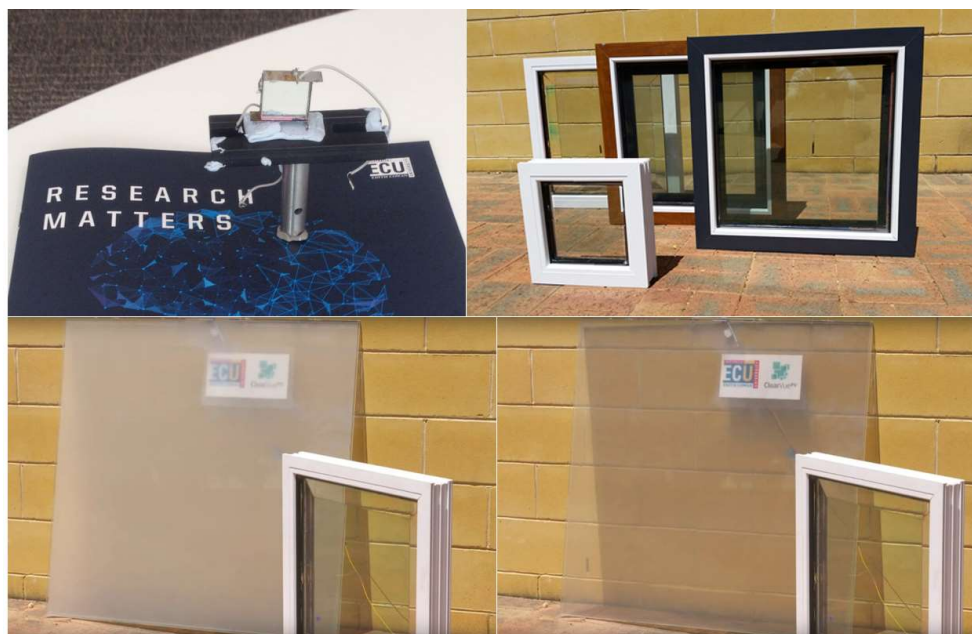
Figure 6. Solar window prototypes and demonstration experiments aimed at the visualisation of energy generation and use conducted at Edith Cowan University (ECU), Joondalup Campus (Perth, Australia), in 2016. A highly transparent framed BIPV window prototype of glass panel dimensions 500mm × 500mm was used to actively change the transparency state of a glass-integrated polymer-dispersed liquid crystal (PDLC) panel of 1m 2 area [47]. .
