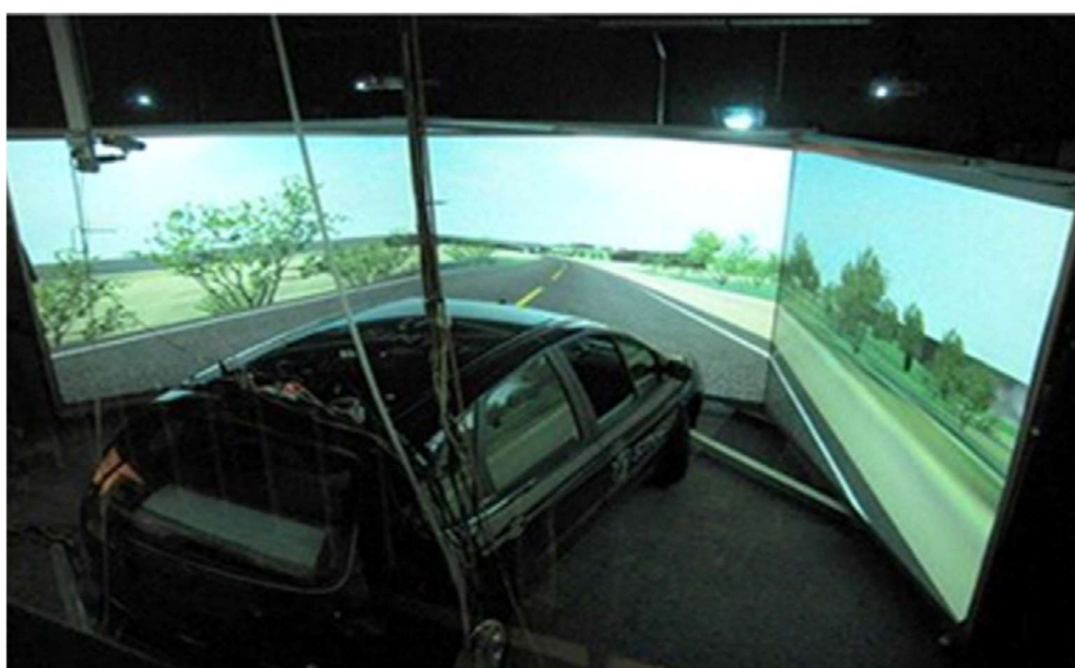
Figura 1.7. Simulatore di guida adottato per l'esperimento "Comparison of driving simulator performance with real driving after alcohol intake A randomised, single blind, placebo-controlled, cross-over trial" (Helland et al., 2013)
