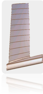
Fig 5.The optimized blade shape of the compressor test rig
