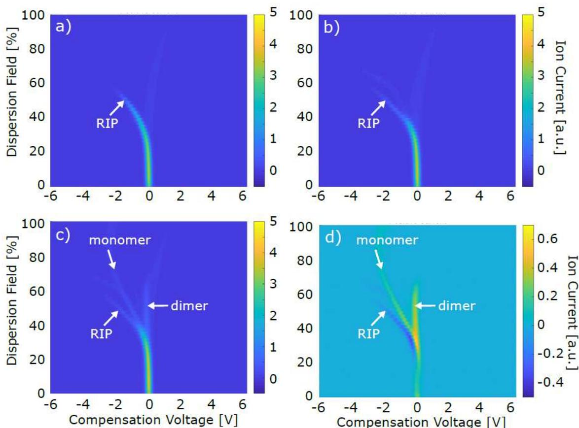
Figure 2. FAIMS dispersion plots. (a) pure air sample (b) CO<sub>2</sub>/air sample (c) acetone/CO<sub>2</sub>/air sample (d) background subtracted acetone/CO<sub>2</sub>/air sample ((c) minus (b)). CO<sub>2</sub> and acetone concentration of these exemplary data were 4 % and 1 ppb, respectively. For the sake of clarity, not all four graphs wear all three axes labels.
