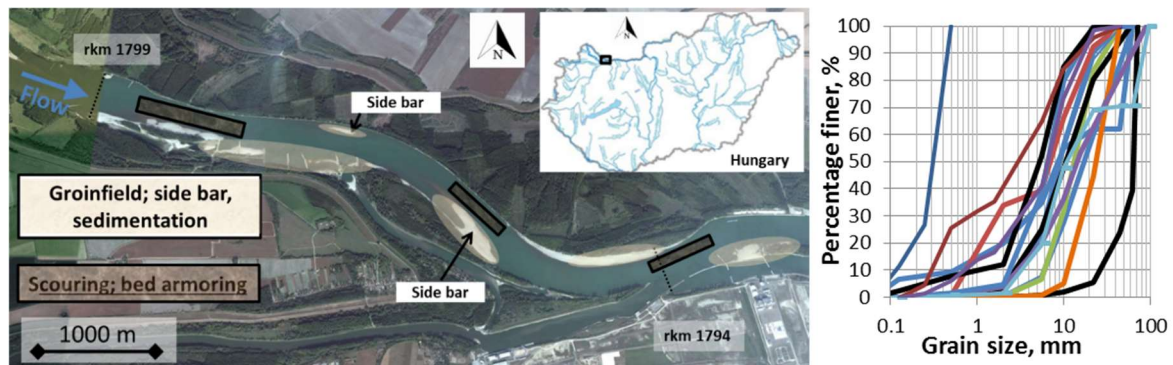
Figure 1. The sketch of the investigated Danube study reach (left) and grain size distributions taken from the investigated reach (right). The characteristic water discharges are Q_m = 2000 \text{ m}^3/\text{s} (mean flow), Q_{bf} = 4300 - 4500 \text{ m}^3/\text{s} (range of bankfull discharge) Q_2 = 5950 \text{ m}^3/\text{s} , Q_{10} = 7950 \text{ m}^3/\text{s} and Q_{100} = 10400 \text{ m}^3/\text{s} (2-, 10- and 100-year flood event) [19].
