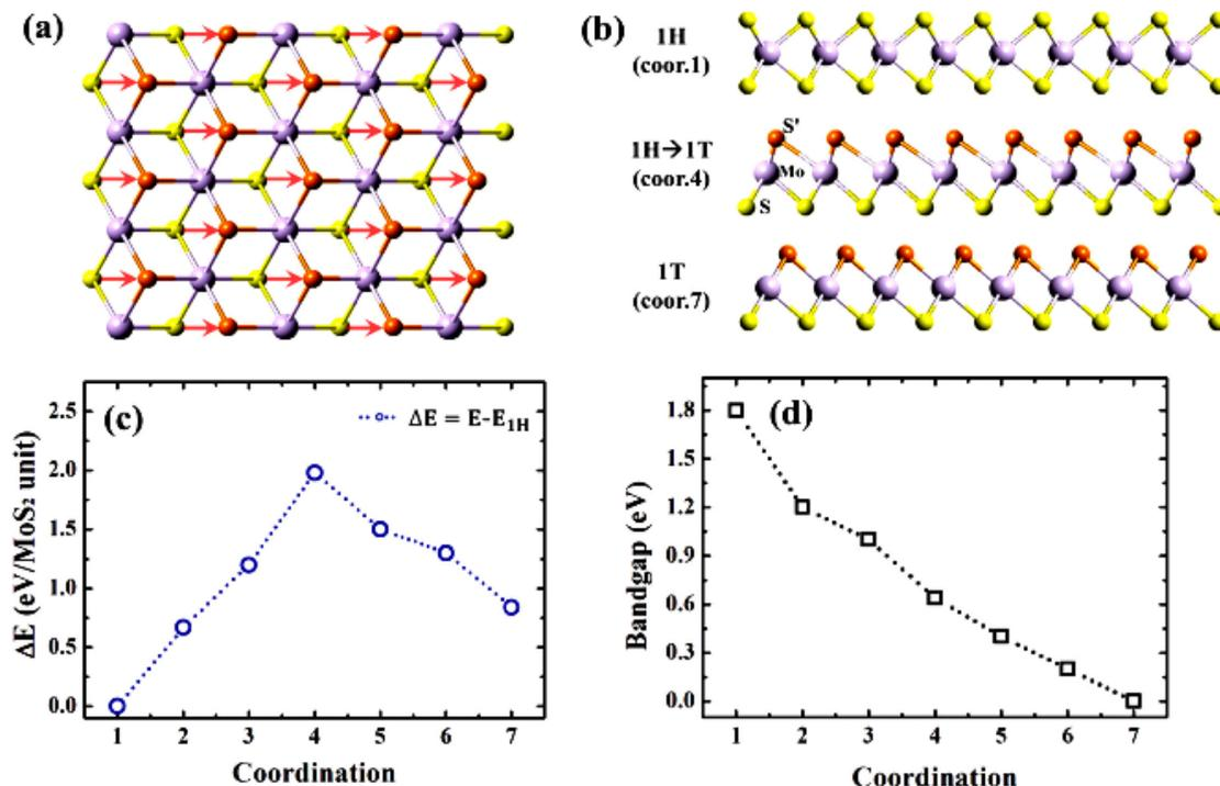
**Figure 1.** (a) Large sphere represents Mo, small yellow and orange spheres represent S and moved S (S'), respectively. Red arrows express moving path of S' atoms. (b) 1H, center of 1H  $\rightarrow$  1T path and 1T correspond to coord.1, 4 and 7, respectively. (c) Energy difference ( $\Delta E = E - E_{1H}$ ) and (d) band gap on the path of the 1H  $\rightarrow$  1T phase transition.
