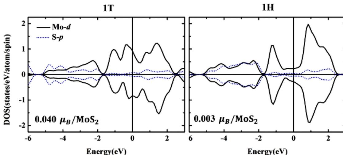
**Figure 4.** Spin-polarized orbital-projected density of state (DOS) of the local 1T phase  $\text{MoS}_2$ . Left panel represents the Mo- $d$  and  $S'$ - $p$  orbital in 1T and right panel does the Mo- $d$  and S- $p$  orbital in the nearest neighbor 1H to  $S'$ .
