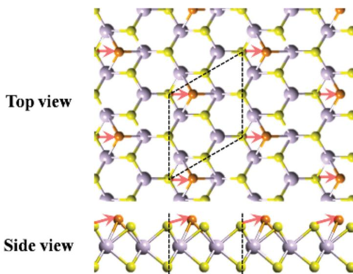
**Figure 2.** Atomic structure of the local 1T phase MoS<sub>2</sub>. Upper (bottom) panel represents top-view (side-view). Dotted lines in both upper and under panels represent the unit cell of the local 1T phase. The moving path of the S' atom is schematically denoted by red arrows.
