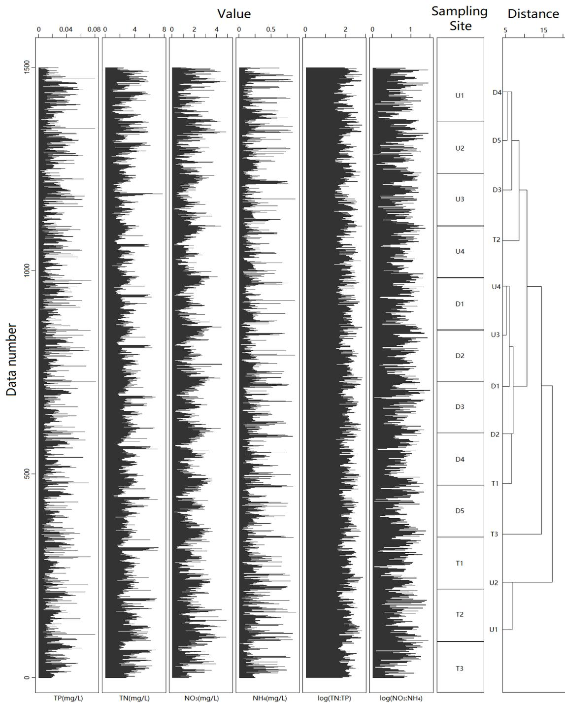
**Fig.3.** Spatial distribution and hierarchical cluster analysis result of water quality parameters in Pingqiao River Catchment. Note: U1 to U4 refer to upstream sampling sites, D1 to D5 refer to downstream sampling sites, and T1 to T3 refer to tributary sites.
