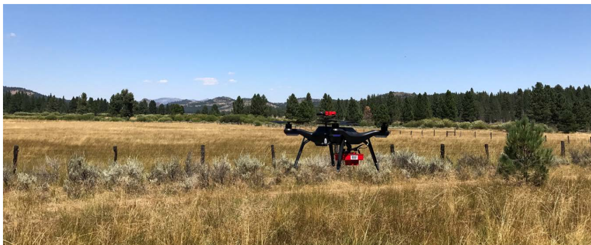
Figure 5. MicaSense RedEdge 5-band camera mounted on a 3DR Solo quadcopter, at lower Knuthson Meadow. This small drone (26 cm width) is capable of carrying a small camera such as a GoPro, or the 150-g MicaSense unit as shown here. Photograph by Quentin Clark, and used with permission.
