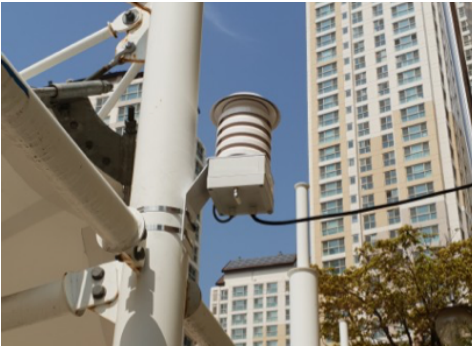
Figure 3. TEOM-based PM sensor.
