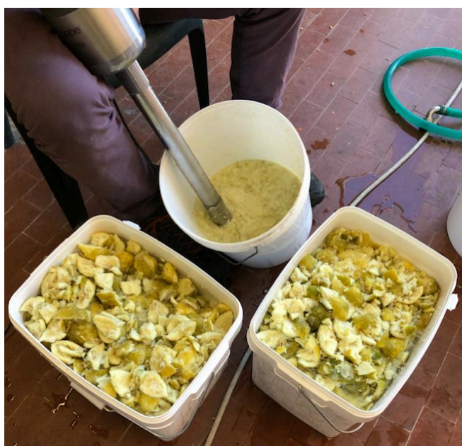
Figure 1. Lemon pectin obtained after freeze drying (top), and waste lemon peel undergoing grinding with a blender prior to the hydrocavitation-assisted extraction process (bottom).
