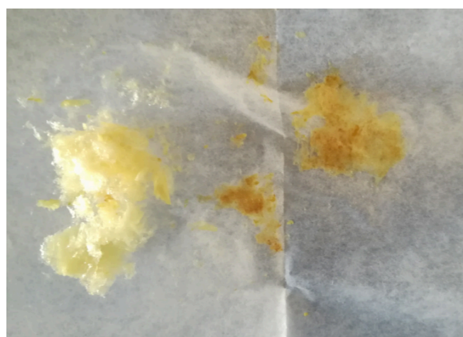
Figure 2. Integral lemon pectin obtained via hydrodynamic cavitation of waste lemon peel (Int-Pec, left), and after thermal treatment at 200°C for 5 min (Int-Pec-Hs, right).
