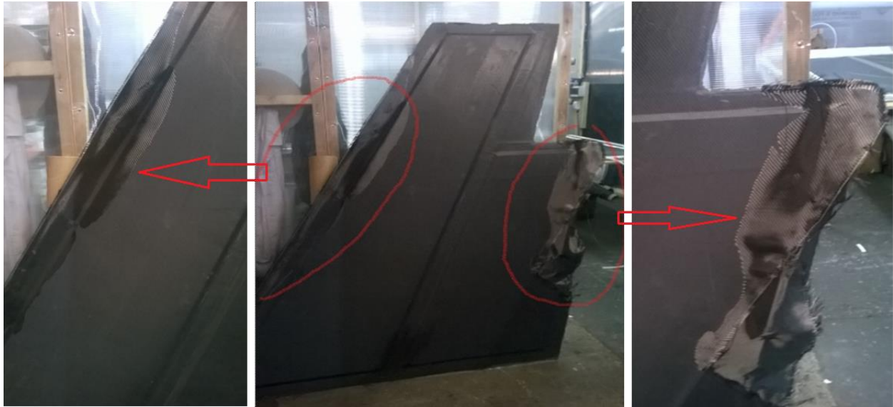
Figure 10. The non-impregnated edges of the cured tail panel in its corners (right) and on the periphery (left)
