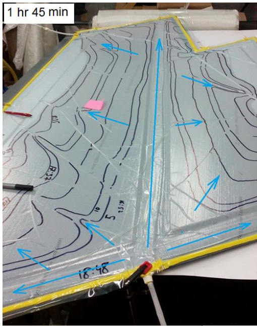
Figure 9. The resin front positions during the vacuum infusion of the tail sandwich panel
