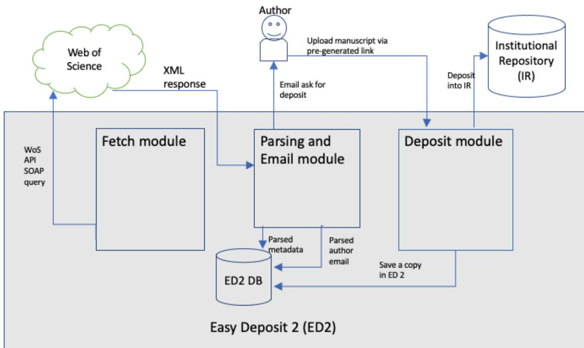
Figure 1. ED2 System Diagram
