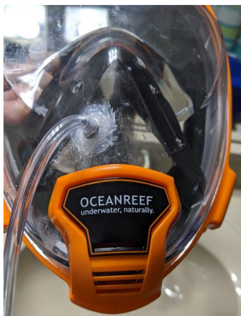
Figure 2. Metal grommet covered with silicone on its outside and inside flat surfaces and extending beyond the grommet's edge to eliminate potential air leaks. Air sampling is inside the mouth/nose compartment. The PortaCount's testing clear tube was secured with superglue.
