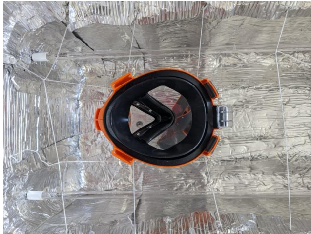
Figure 6. Snorkel mask inside UVC light box.
