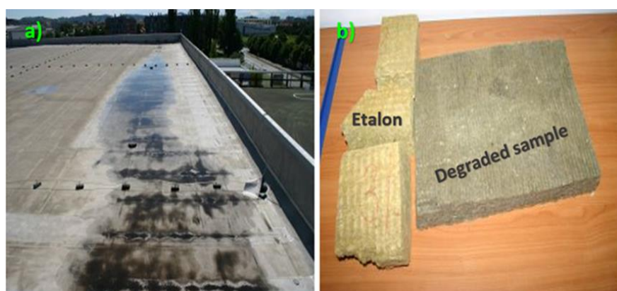
Figure 2. (a) Mineral wool samples taken from softened, uneven roofing areas of a commercial building located in Slovenia, central Europe. (b) Visual presentation of new and degraded insulation samples
