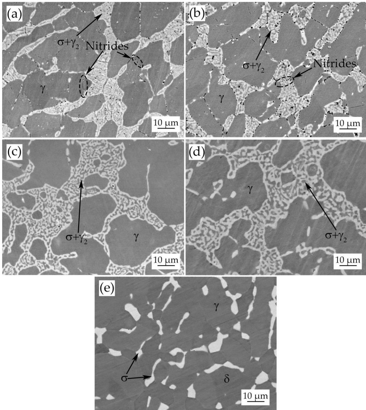
**Figure 5.** Microstructure after 24 hour heat treatment at: 850 °C (a), 900 °C (b), 950 °C (c), 1000 °C (d) and 1050 °C (e).
