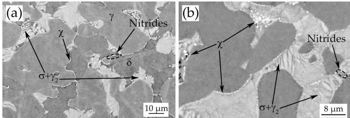
**Figure 2.** Microstructure after heat treatment at 850 °C for: 10 min (a) and 25 min (b).
