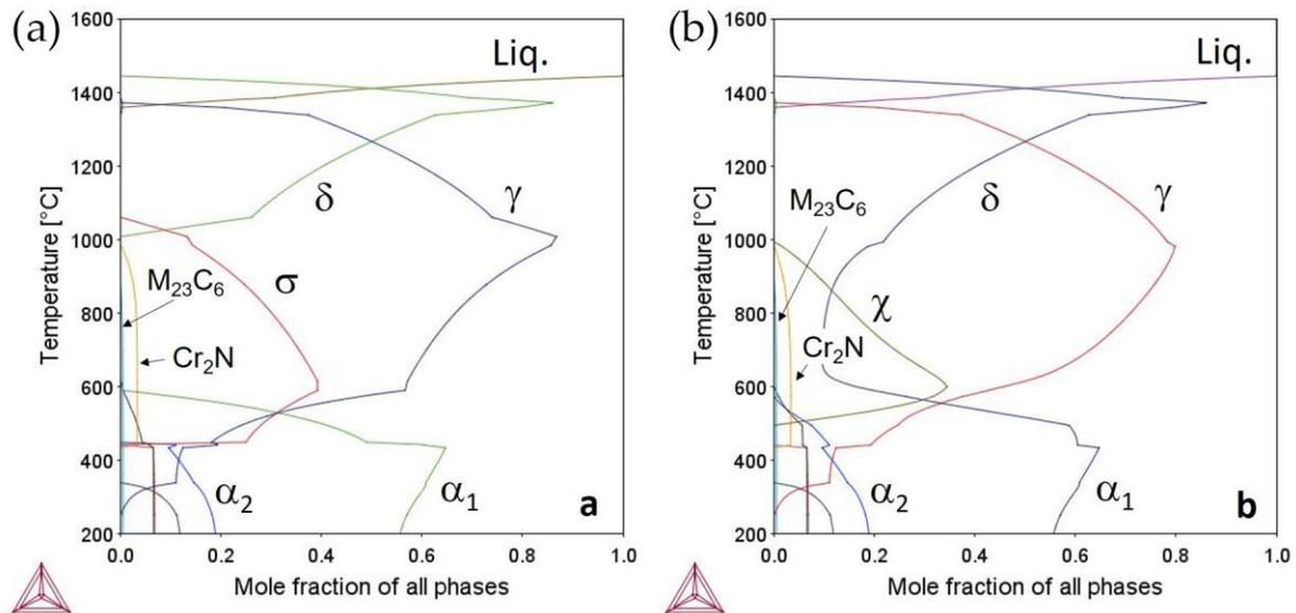
**Figure 1.** Property diagrams showing the mole fraction of phases vs. temperature under equilibrium conditions (a) and after suppressing  $\sigma$ -phase formation (b).
