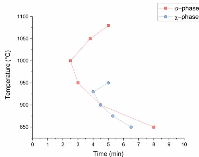
**Figure 6.** First observed appearance of  $\sigma$ -phase and  $\chi$ -phase (approximately 0.1%)
