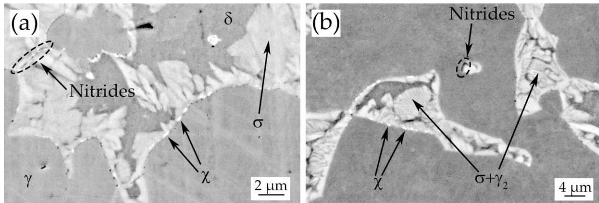
**Figure 3.** Microstructure after heat treatment at 900 °C 5 min (a), 950 °C 15 min (b)
