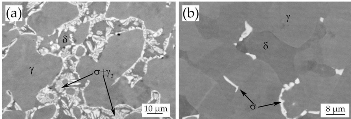
**Figure 4.** Microstructure after heat treatment at 1000 °C 3 min (a), 1080 °C 10 min (b)
