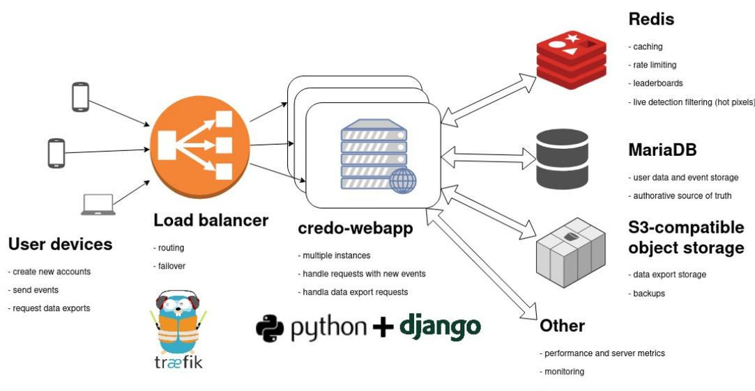
Figure 17. Diagram representing the architecture of storage application.
