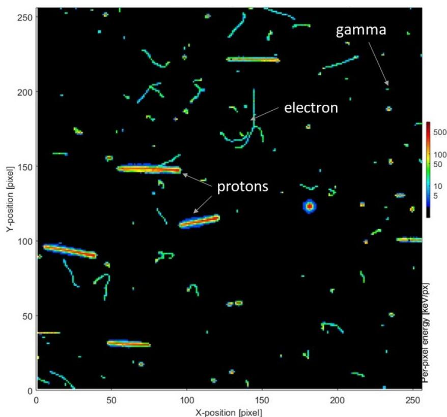
**Figure 12.** An example of per-pixel energy deposited by various particles in a mixed radiation field measured using a Minipix Timepix detector with Silicone sensor. The detector was operated in ToT-frame mode with an acquisition time of 10 ms. Low-energy, narrow, curly tracks are typical for electrons, high-energy, wide, straight tracks for energetic heavy charged particles such as protons.
