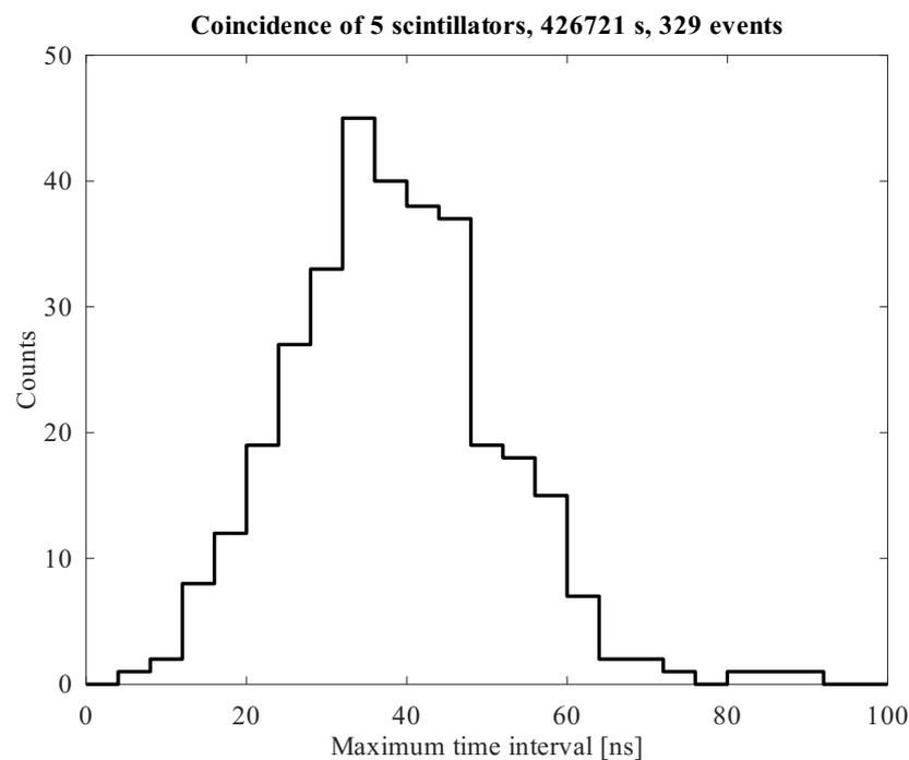
**Figure 13.** Distribution of maximum time intervals of 329 events of five-fold coincidences registered by spectrometer's active shield during single gamma-ray spectrometry measurement (time of measurement 426721 s).
