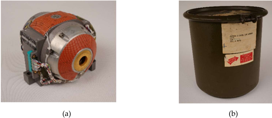
Figure 25. The Gyro G200 of the LN3 Inertial Platform: (a) Gyro G200; (b) G200 transportation box
