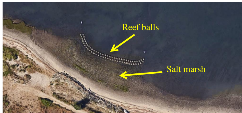
Figure 11: Ecological- based coastal protection system in Short Beach. Since setting up the protection system, sediment erosion has stopped and the system successfully trapped sand and finer sediment
