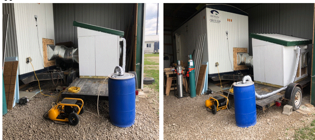
Figure A1. Picture of UV mobile laboratory (back) and filter house mounted on a trailer (front) with manure drum and gaseous emission generation system.
