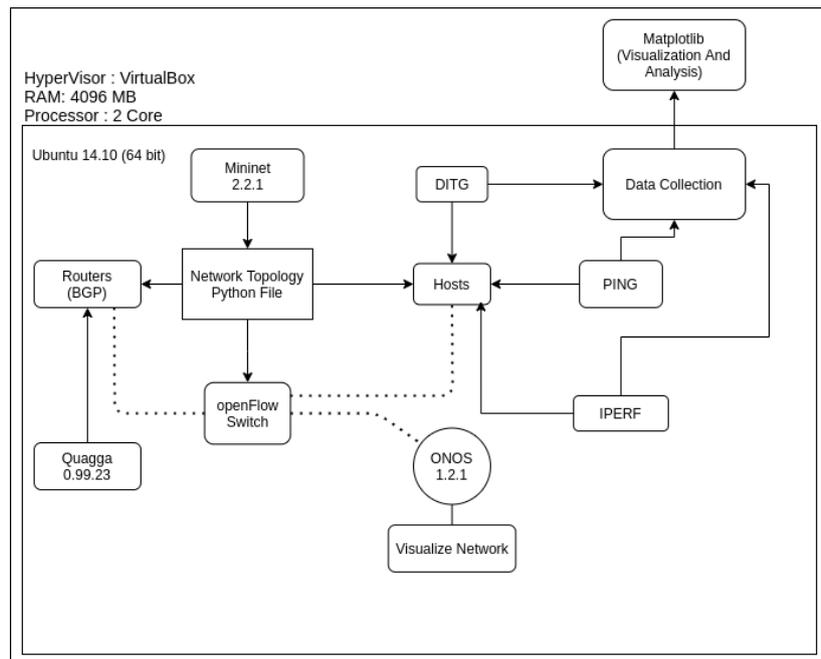
**Figure 4.** System setup simulation environment
