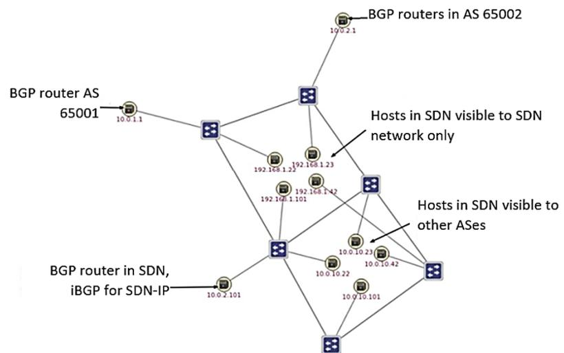
**Figure 2.** Experimental topology of SDN integrated with Legacy networks
