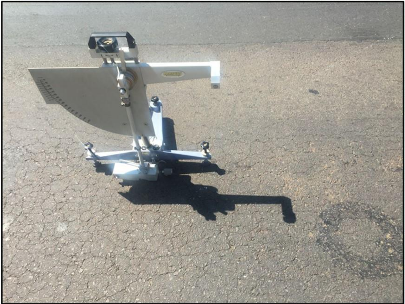
Figure 10: Skid resistance testing done before and after application of a clear-seal [23]
