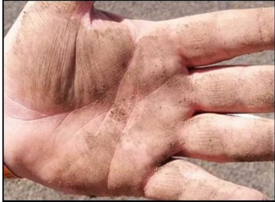
Figure 12: Demonstration of the effect of the organofunctional modification of the anionic bitumen emulsion used in the NME pot-hole kits that is designed to adhere to granular material, resulting in a minimum contamination when in contact with bare skin
