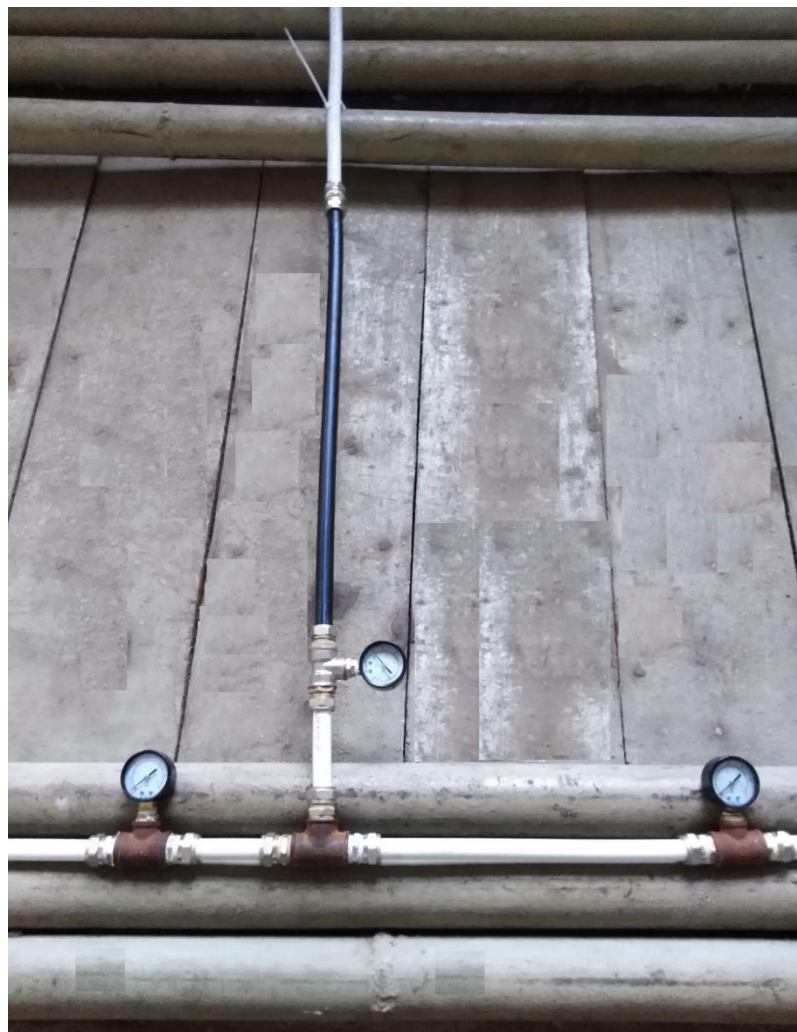
Figure 3. Determination of local head loss in equal-pass T-Junction at flow division at angle \alpha = 90^\circ .
