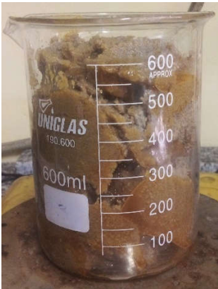
Figure 2. Pre-treated residual fat used as feed material by catalytic upgrading of residual fat vapors at 400 °C, 1.0 atm, 0.0, 5.0, 7.5, and 10.0% (wt.) activated carbon pellets impregnated with 10.0 M NaOH, using a catalyst fixed bed reactor, in semi pilot scale.
