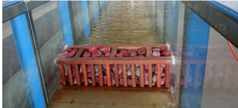
Figure 5. Experimental pile-rock breakwater set up in the wave flume in the laboratory.
