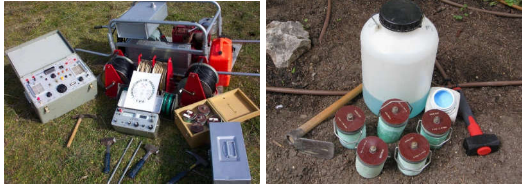
Figure 2. (a) Scintrex TSQ-3 equipment and IPR-10A receiver. (b) Fat non-polarisable electrodes with \text{CuSO}_4 .
