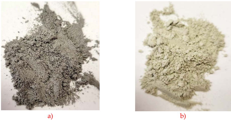
Figure 1. Appearance of the fillers used: a) Fly ash from the SDPP; b) Backfill material obtained from the mineral processing waste of the copper-mining plant
