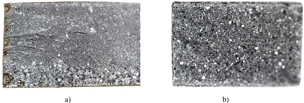
Figure 14. Photo of cross-sections of filled specimens: a) EP-FA25; b) EP-FA50
