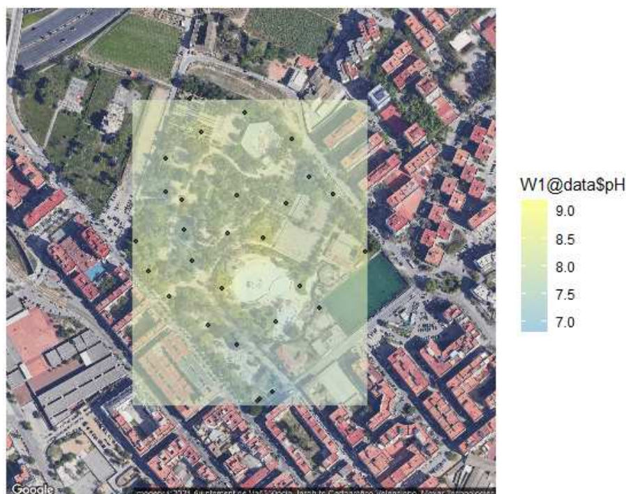
Figure 2. Kriging distribution of pH measurements (black dots) at the Park of Benicalap.
