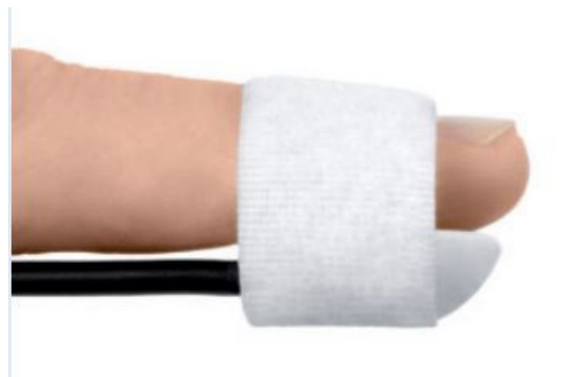
Figure 1. Example of dual PES/PCS sensor affixed to the index finger.
