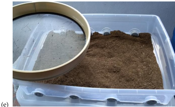
Figure 4. (a) Fresh organic manure (90 % moisture) in the 150-L stabilization chamber; (b) CaCl 2 in the tray of the condensation vessel; (c) stabilized manure after 2 weeks of operation (45 % moisture); (d) testing the CaCl 2 -brine as additive of fresh slurry, which was generated in the condensate chamber, to avoid crust formation; (e) upgraded soil organic amendment (25 % moisture) after 2-mm sieving.
