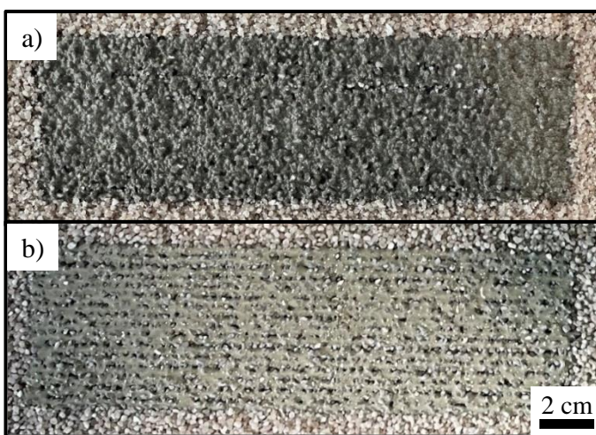
Figure 7: Comparison of cement paste penetration for aggregates: a) standard aggregates without dry water; b) aggregates mixed with dry water
