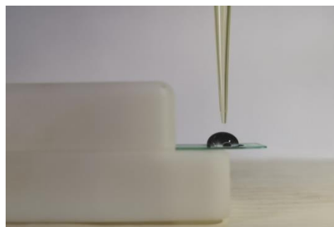
Figure S9. The photo of commercial screen-printed microelectrode with a drop of solution containing nitrite (200 \mu\text{L} ).
