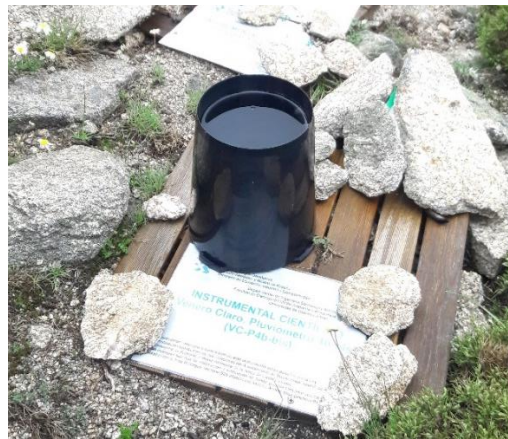
Figure 4. Clogged TBR with rainfall water accumulated in the funnel (IGME, Venero Claro, Spain).
