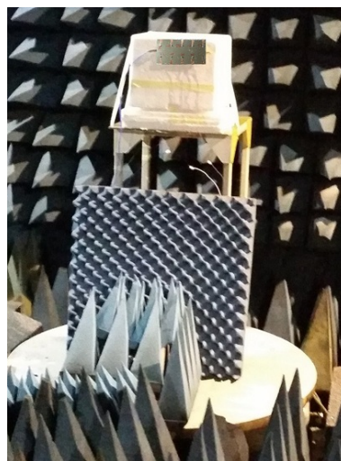
Figure 12. Measurement Setup of a Proposed Antenna
