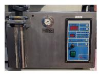
Figure 2. Hydrogen welder.
