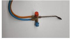
Figure 1. Gas welding torch.
