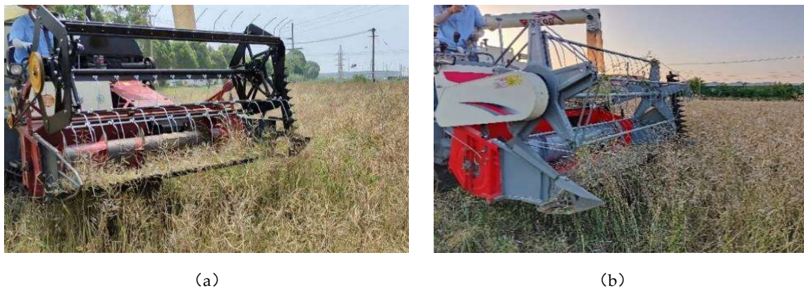
Figure 6. Comparative test of two types of reel cutting tables. (a) Variable speed reel, (b) Cam-action reel.
