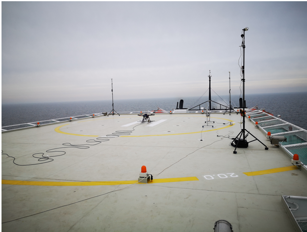
Figure 3. Tethered hexarotor with other UAS components on the ferry's top deck
