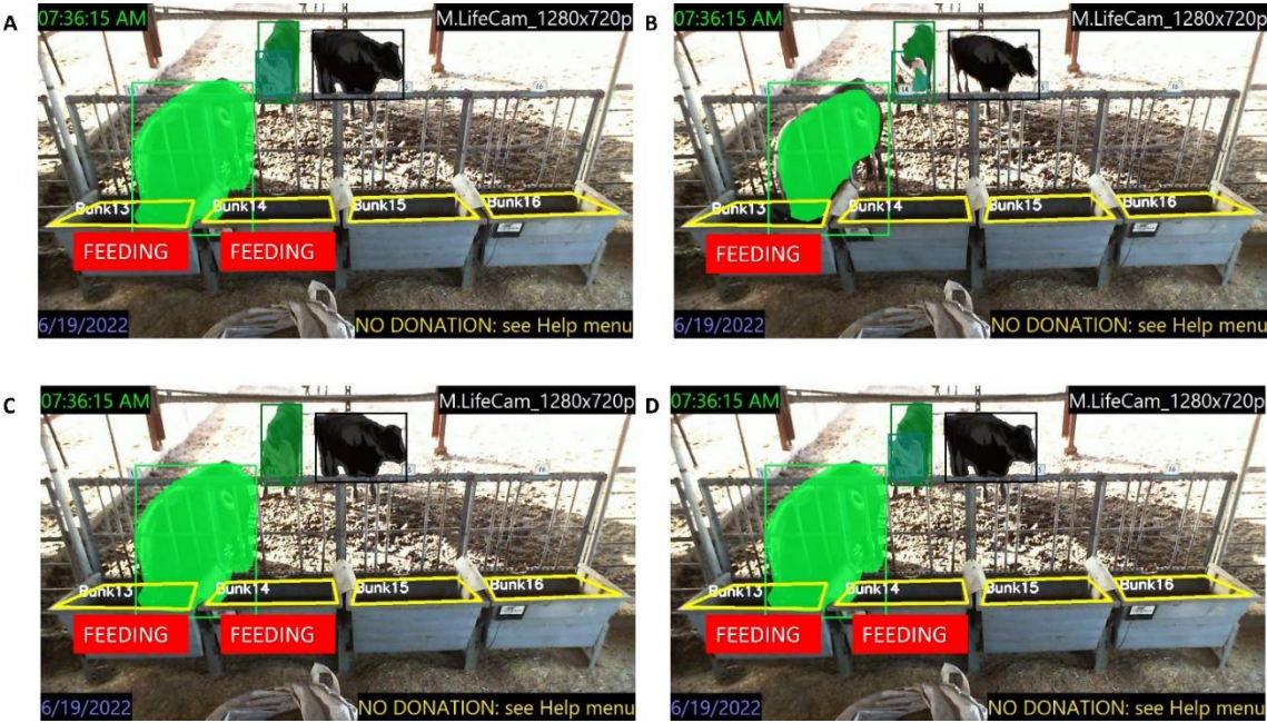
Figure 5. Pixel segmentation examples using different mask and box thresholds. (A) Mask 0.1 and box 0.1. (B) Mask 0.9 and box 0.1. (C) Mask 0.1 and box 0.9. (D) Mask 0.9 and box 0.9.
