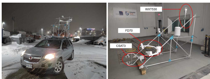
Figure 2. The WoW vehicle used for field measurements [15].
