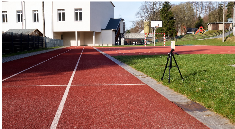
Figure 3. Our camera-based photoelectric barrier can be easily placed on a tripod. Unlike traditional systems, we don't require a reflector, which greatly reduces setup time. Bluetooth communication eliminates the need for wires.
