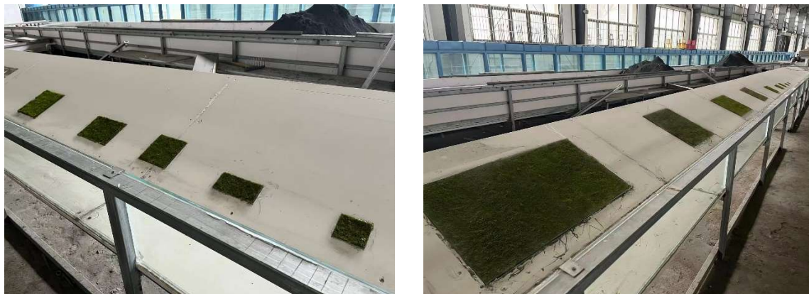
Figure 4. Distribution of epipellic algae clusters of different sheet sizes on the side wall.
