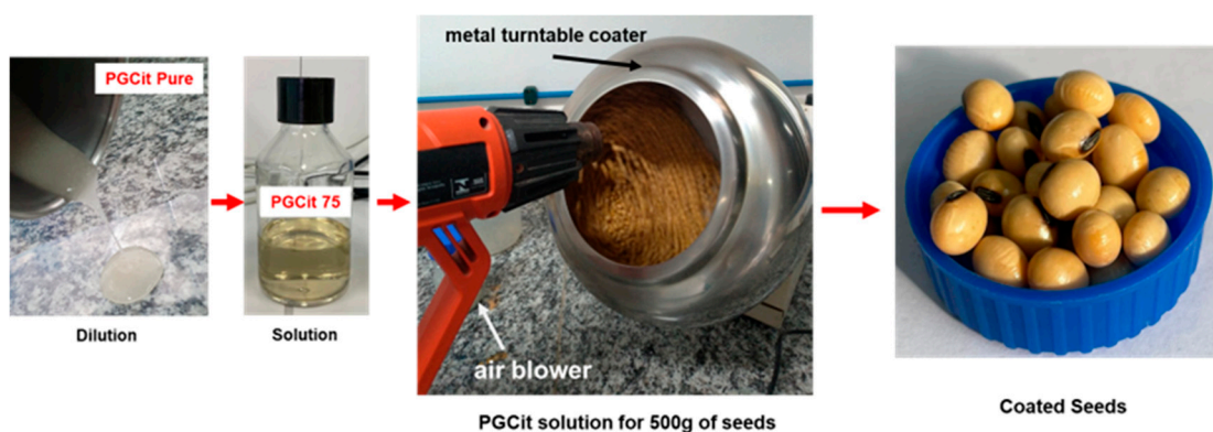
Figure 11. Soybean coating procedure with PGCit polymers.
