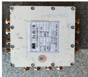
Figure 10. our developed ECU of intelligent chassis with explosion-proof processing.
