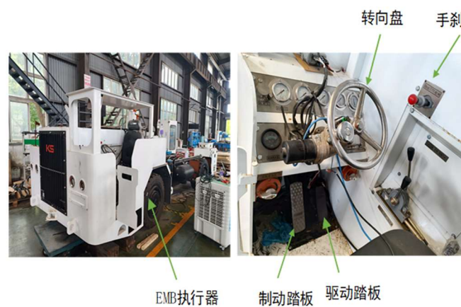
Figure 11. Experimental setup. (a) proposed EMB system block diagram; (b) test vehicle equipped with designed EMB.
