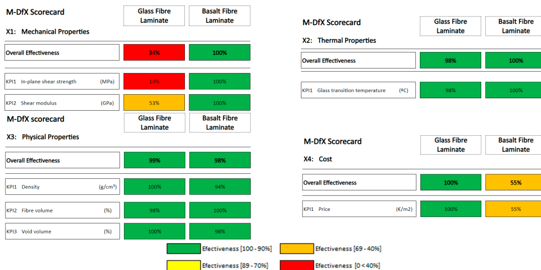
Figure 4. M-DfX Scorecards Effectiveness for the glass and basalt laminates.
