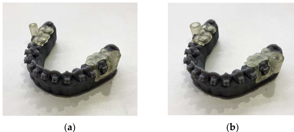
Figure 17. (a) is the predrilling surgical guides; (b) is the TADs surgical guides.
