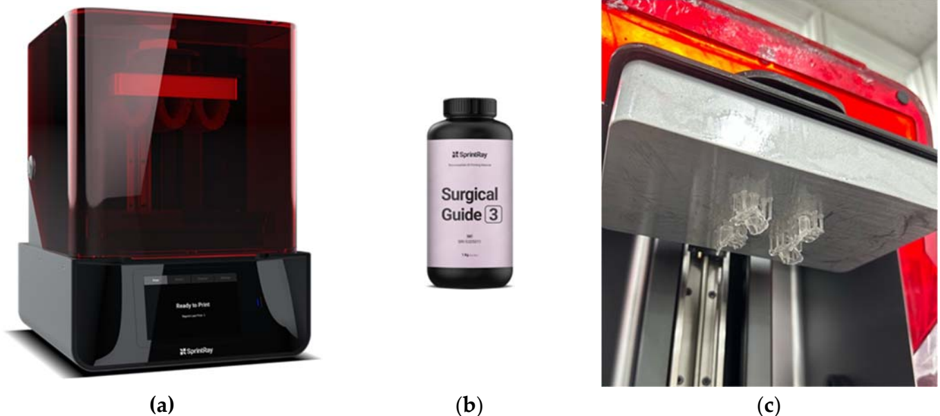
Figure 14. (a) is the printing machine; (b) is the acrylic substance; (c) is the printing result
