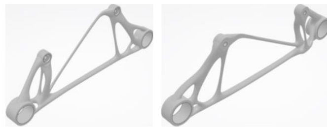
Figure 17. Final design of the optimized front electric motor holder.
