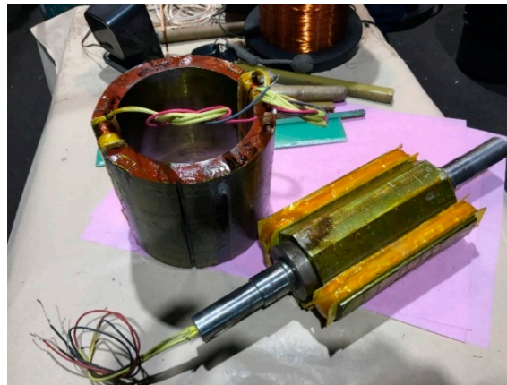
Figure 7. AC/DC rotating current sensor during manufacturing.
